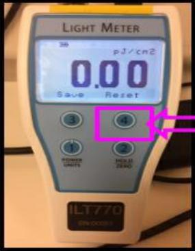
Select button "4" to reset meter to zero
